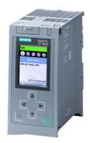
\*\*\*Spare part\*\*\* SIMATIC S7-1500, CPU 1515-2 PN, Central processing unit with work memory 500 KB for Program and 3 MB for data, 1st interface, PROFINET IRT with 2-port switch, 2nd interface, Ethernet, 30 ns bit performance, SIMATIC Memory Card required
